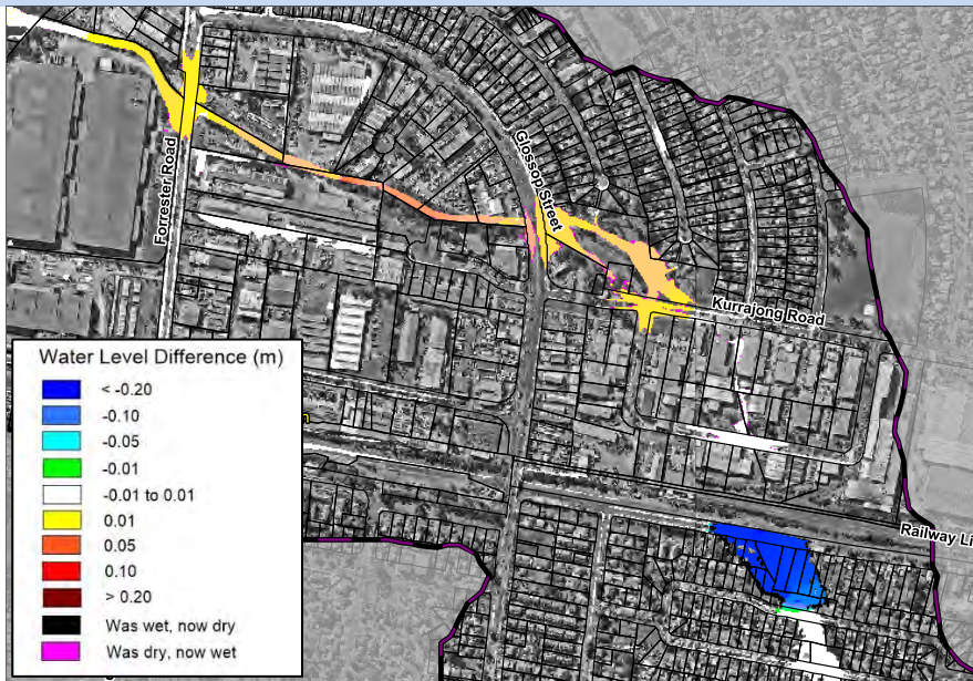
Plate 23 Flood Level Difference Maps for FM2
