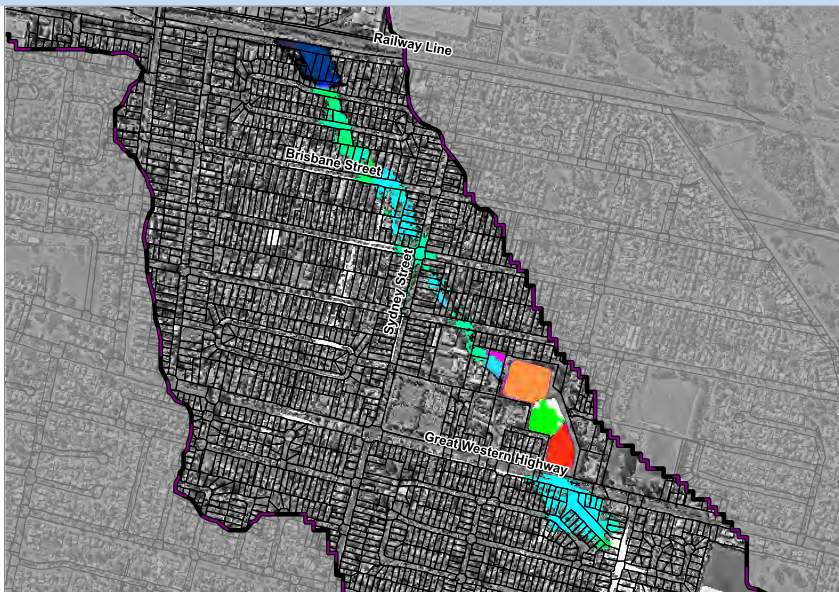
Plate 37 Flood Level Difference Maps for FM10
