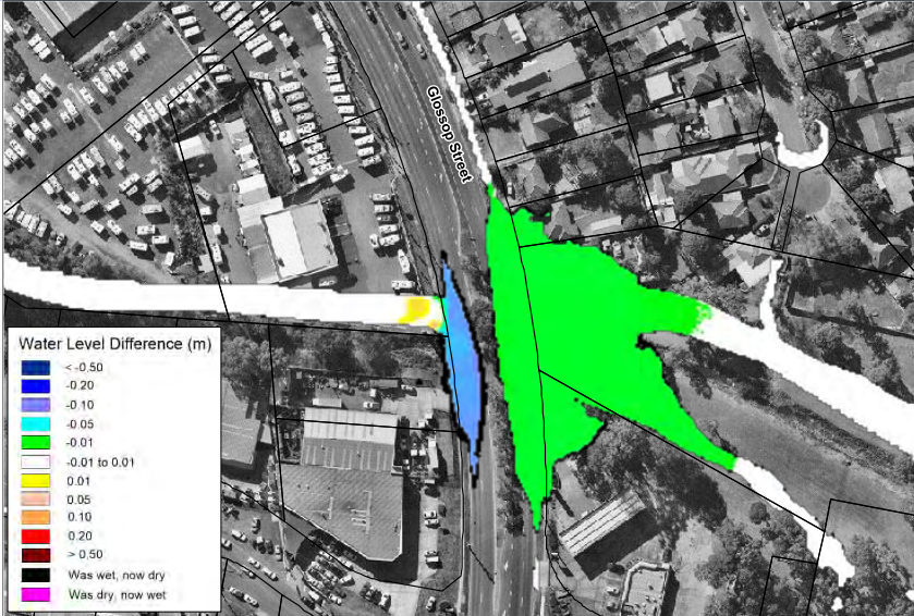
Plate 29 Flood Level Difference Maps for FM5
