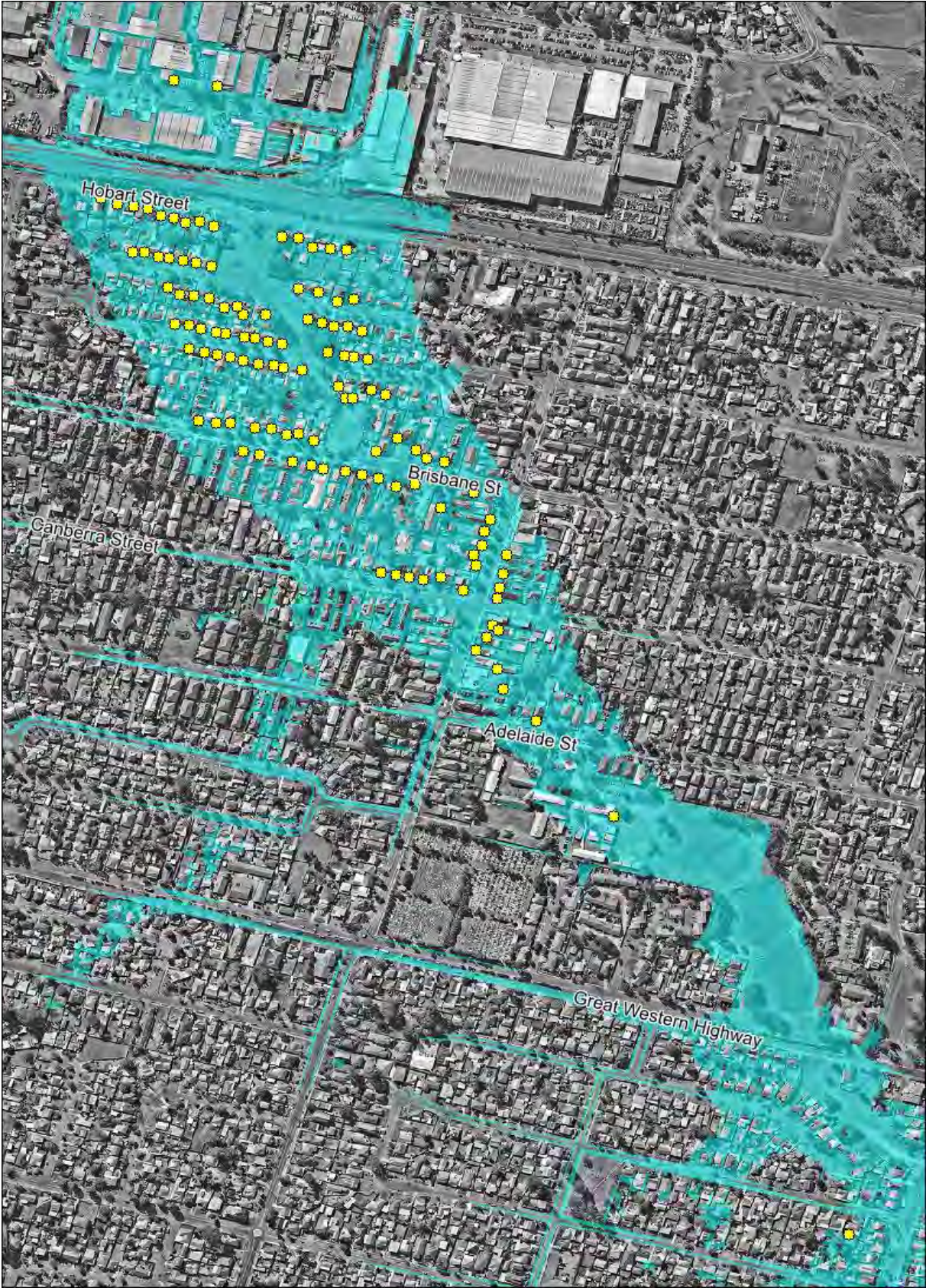
Plate 19- Properties estimated to have flood depths above floor level greater than 1.2 meters in the PMF (evacuation considered essential).
