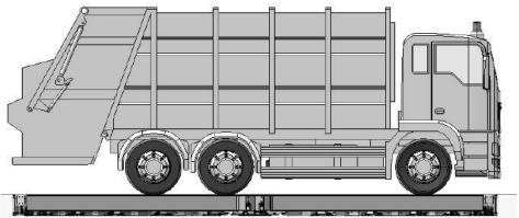
Figure 6: Correct vehicle loading alignment showing central alignment and no vehicle overhang
