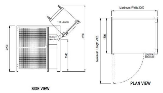
Figure 47: 1100L bin lifter schematic side and plan view
