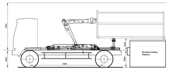
Figure 29: Hook Lift Vehicle ground loading configuration
