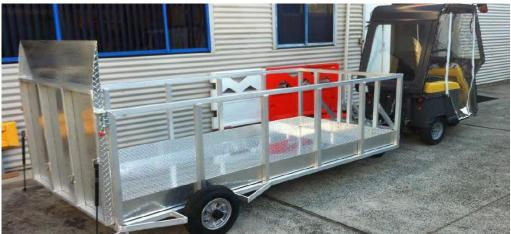
Figure 18: Aluminium Trailer attached to an Electric Tug Device
