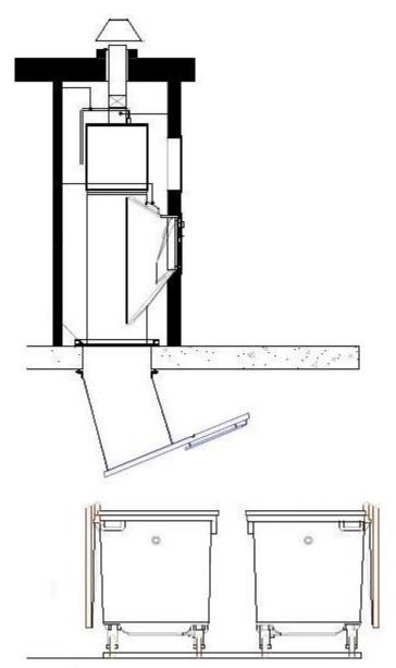
Figure 27: Cross section of a chute inlet throughout various level of the building
