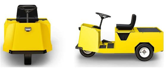
Figure 11: Typical Electric Ride On Tug Device used by the caretaker for the movement of 660L & 1100L bins within the development
