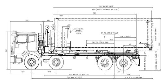
Figure 48: 9.1m Hook Lift Waste Collection Vehicle specifications
