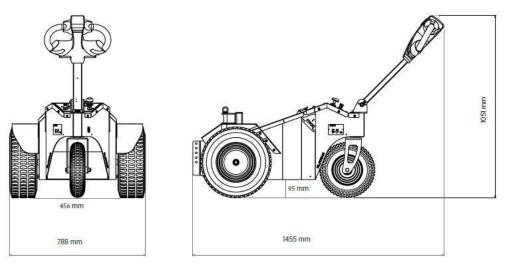
Figure 20: Schematic of a typical Portable Bin Tug Device
