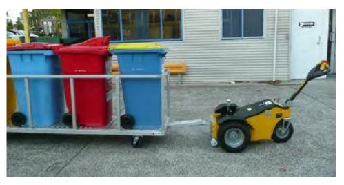
Figure 22: Portable Bin Tug Device moving bins using an aluminium trailer
