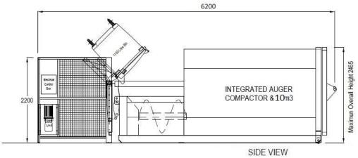
Figure 37: 6.0m Integrated Auger schematic side view
