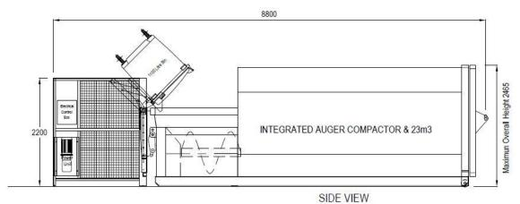
Figure 52: 7.0m Integrated Auger schematic side view
