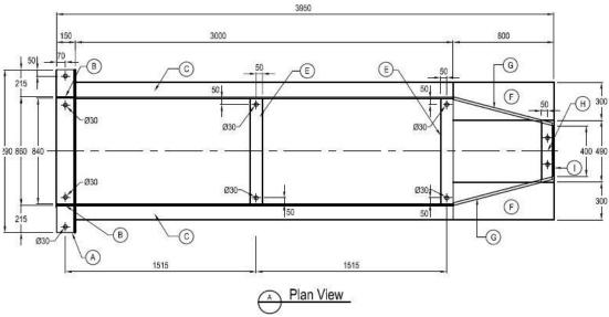
Figure 46: Integrated Auger Guide rails plan view
