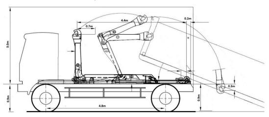
Figure 28: Hook Lift Vehicle ground loading configuration
