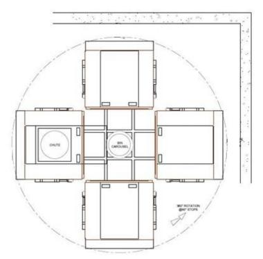
Figure 26: Design configuration of a circular carousel accommodating 1,100L bins
