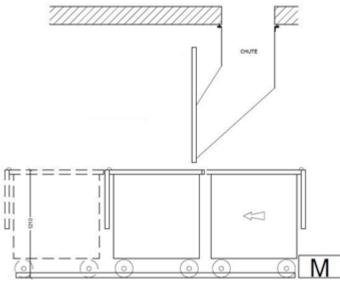
Figure 25: Design configurations of a linear track system accommodating 1,100L bins
