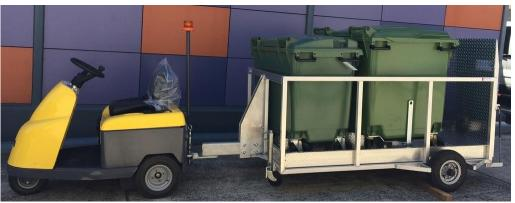
Figure 17: Aluminium Trailer attached to the Electric Tug Device for 660L and 1100L bin movements
