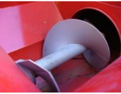
Figure 31: Integrated Auger used to compact objects within the compaction unit
