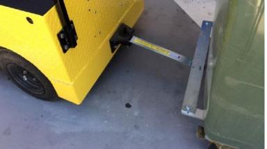
Figure 14: Universal Rowing Device attachment to the Electric Tug Device
