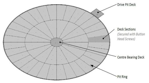
Figure 3: Turntable reference diagram depicting key components and terminology
