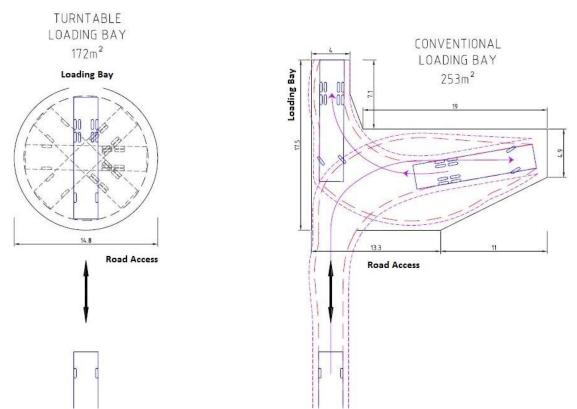
Figure 9: Swept path model showing the area requirements between two loading bay configurations utilising a 12.5m Heavy Rigid Waste Collection Vehicle (AS2890.2)
