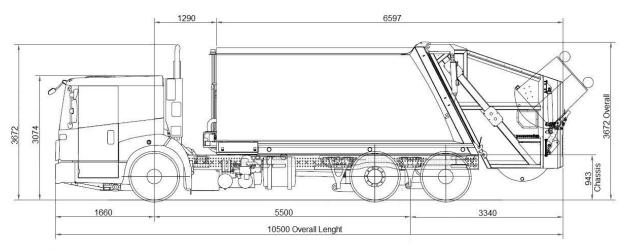
Figure 2: 10.5m Heavy Rigid Rear Load Waste Collection Vehicle specifications
