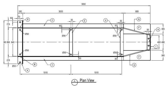
Figure 38: Integrated Auger Guide rails plan view
