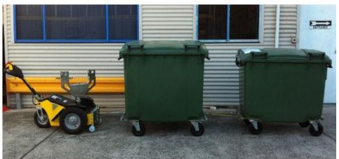
Figure 21: Portable Bin Tug Device moving 1100L bins in a train configuration
