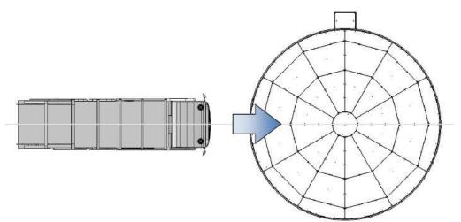
Figure 4: Central alignment of a heavy rigid collection vehicle onto the turntable
