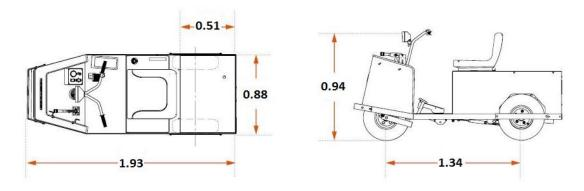
Figure 12: Schematic of a Typical Electric Ride On Tug Device
