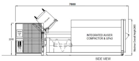
Figure 45: 6.0m Integrated Auger schematic side view
