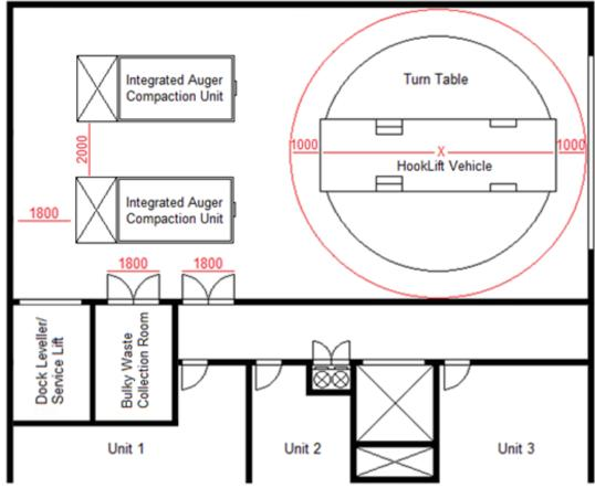
Figure 55: Concept configuration of ground floor waste infrastructure required to service compaction units within Residential Flat Buildings
