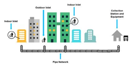
Figure 1: Automated Waste Collection System schematic identifying key infrastructure
