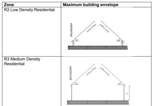
Figure D2.10: The building envelope is measured from natural ground level perpendicular to the side boundary at any given point along the wall.
