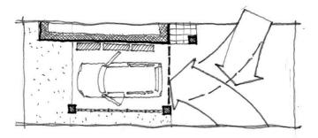
Figure D2.7: Two spaces - one covered plus one open, either stacked or paired
