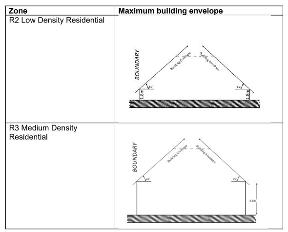
Figure D2.1: The building envelope is measured from natural ground level perpendicular to the side boundary at any given point along the wall.
